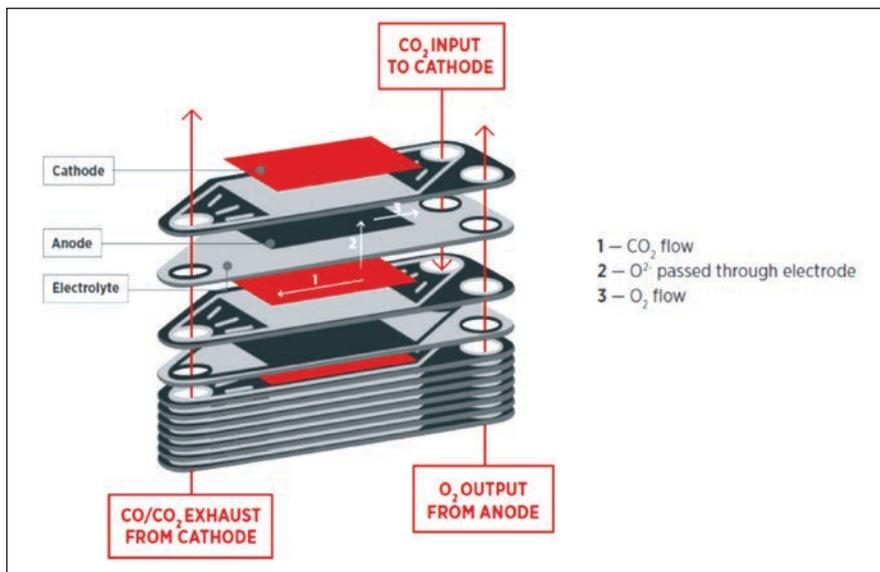
Figure 3. Schematic of electrolysis using SOXE stack.
