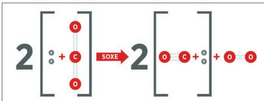
Figure 4. The process of solid oxide electrolysis converts CO<sub>2</sub> to O<sub>2</sub>.
