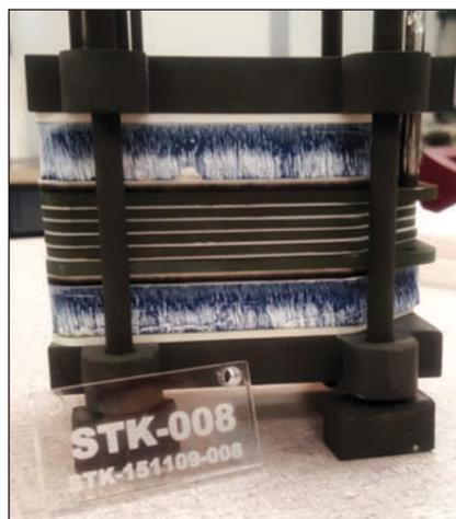
Figure 2. Prototype SOXE stack of ScSZ engineered ceramic electrolytes.
