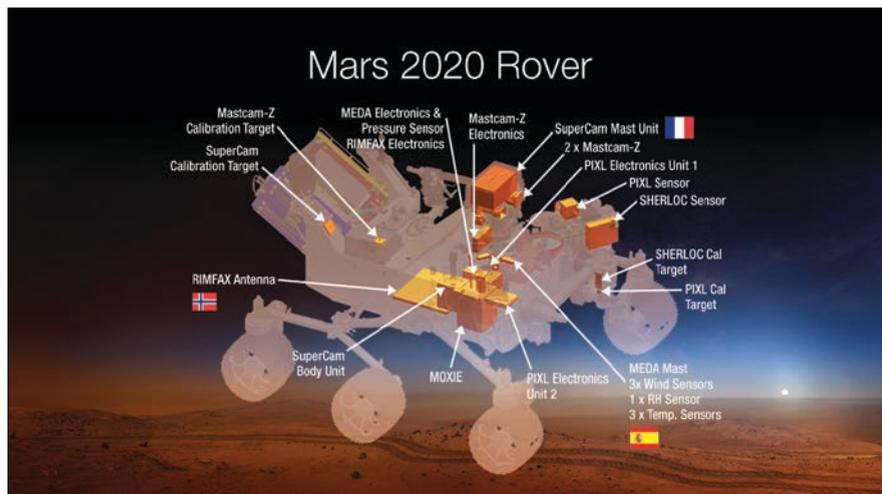
Figure 1. Illustration of planned Mars 2020 Rover incorporating seven instruments, including MOXIE. (Image courtesy of NASA.)
