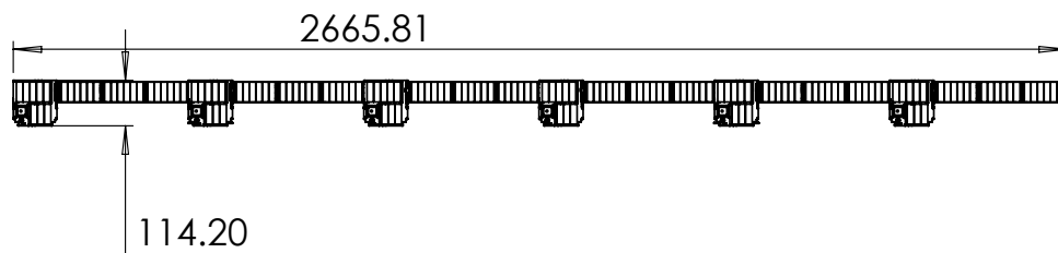
Figure 4 ThinSat 6T Spacecraft, Dimensions in mm
